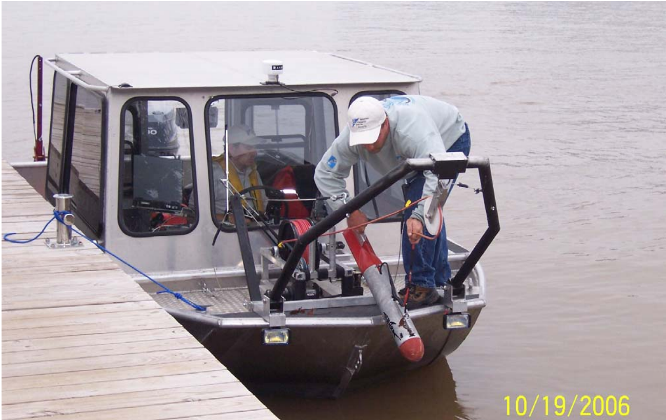
Figure 4.1. Aluminum Survey Boat Used by MCDI for Side-scanning Sonar Surveys. Torpedo-shaped item is the side-scanning sonar transponder.
